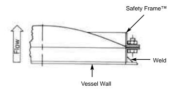
FIG. 2 - VENT-SAF<sup>™</sup> Assembly Welded to the Customer Structure
