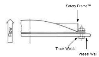
**FIG.1** - VENT-SAF<sup>™</sup> PLUS Assembly Bolted to the Customer Structure
