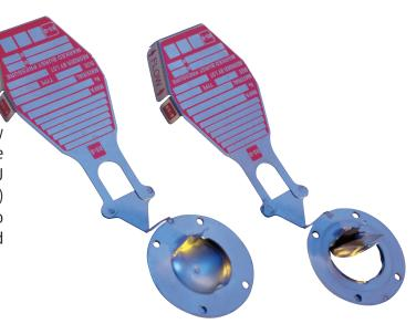
The  $SK_R$ -U is a two-part rupture disk comprising a calibrated metal dome that faces into and responds to a source of overpressure, and a stainless steel hinge ring permanently fitted to the downstream side of the disk that works together with the safety head to retain the disk petal after opening. These pressures are applicable to all sizes of  $SK_R$ -U rupture disk: 1/2, 3/4 and 1 inch. Standard safety head material is 316 stainless steel.
